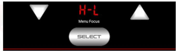
Swiping the control area to the left or right brings the **SR** version of the rotary controls on the subwoofer panel. Each pair of buttons represents a single rotary of the four: **H-L**(high level gain), **Hro** (high level roll off), **LFE**(low level gain) and **Lro**(low level roll off). These controls have exactly the same function as the rotaries on the subwoofer panel. (please see the subwoofer manual for more details)
